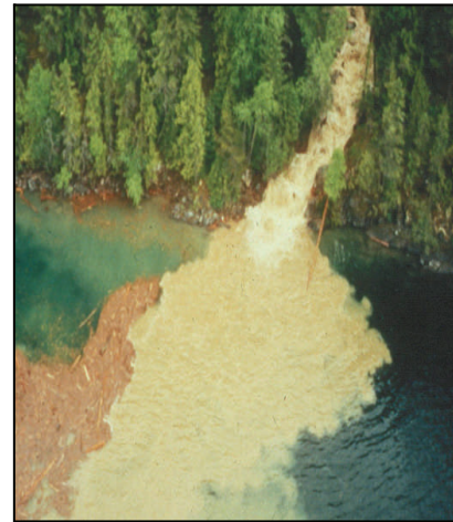
Figure 2. Debris flood on Memphis Creek. Note the large volume of floating debris in the lake and the uncharacteristically turbid water.
